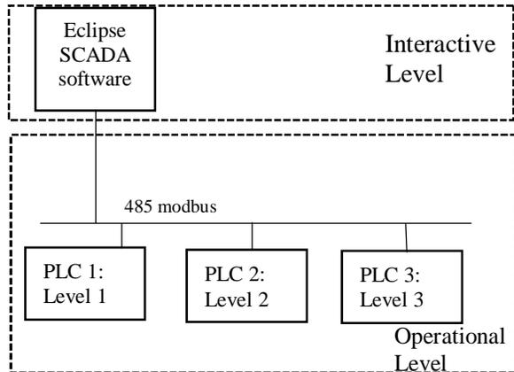
Fig. 1: Supervisory Control Architecture
